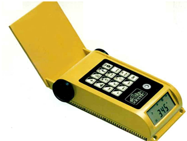
Figure 6: A Clar electronic geological compass manufactured by F.W. Breihapt in Germany.
